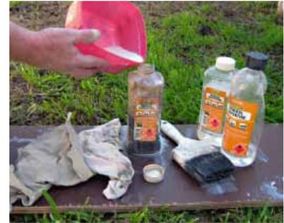
Turpentine is needed for washing equipment that has been used with oil based paints, and can be recycled. It is expensive, and to successfully clean brushes and rollers it is necessary to use at least three lots of turpentine before finally washing in soap and water.
