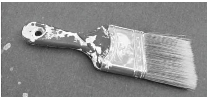
**Typical general brush sizes:** 25–50mm for trim, touch ups, screens, furniture; 50–75mm for doors, beams, shelving, fences; 75–100mm for walls and panelling. Natural bristle brushes are soft and porous, and intended for use with oil based paints. Avoid natural bristle with water based paints.
